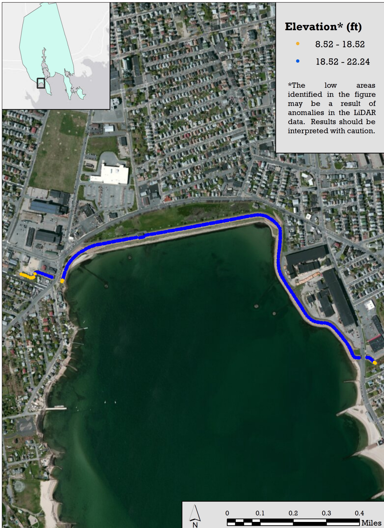
Figure 10. Clarks Cove Dike elevations.
