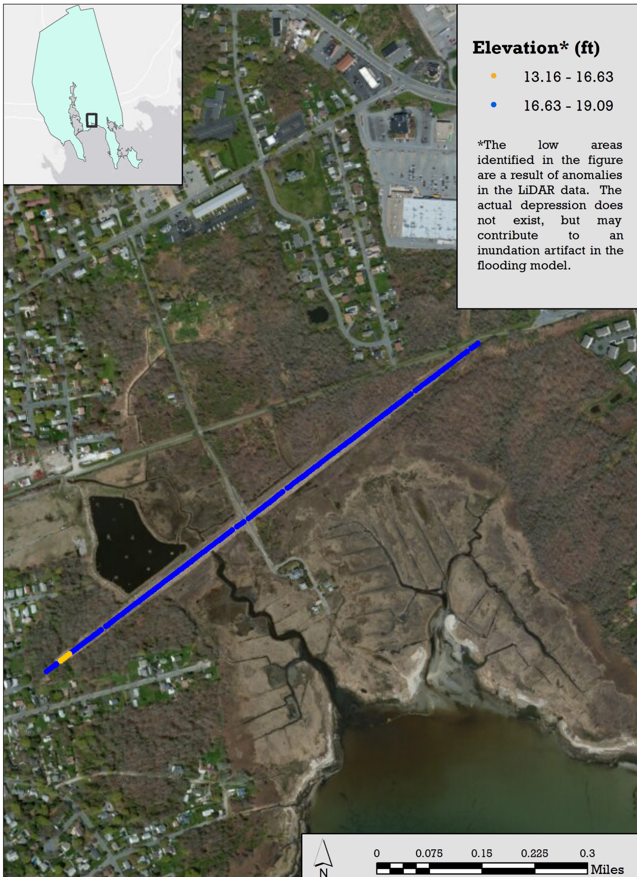
Figure 11. Fairhaven Dike elevations.
