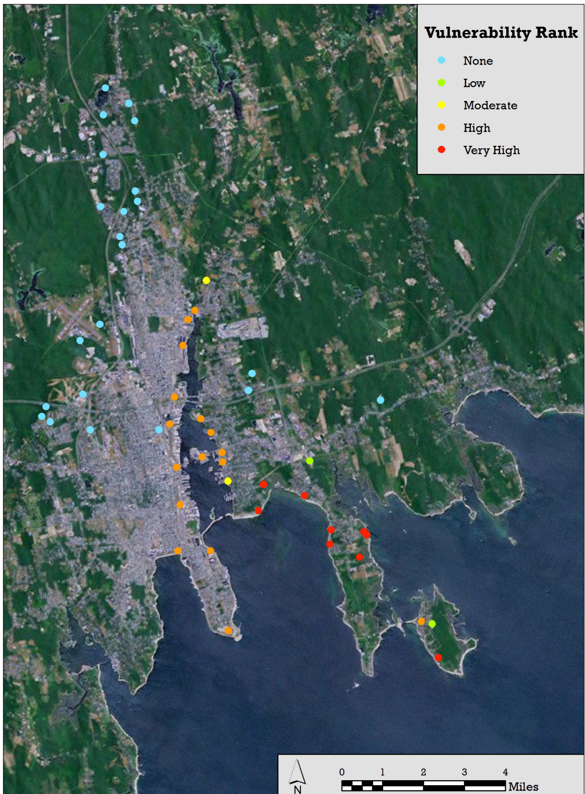
Figure 19. Outfalls by vulnerability rank. If the outfall is vulnerable in 1-5 storm scenarios, it is given a risk ranking of low and colored green. If the outfall is vulnerable in 6-10 storm scenarios, it is given a risk ranking of moderate and colored yellow.
